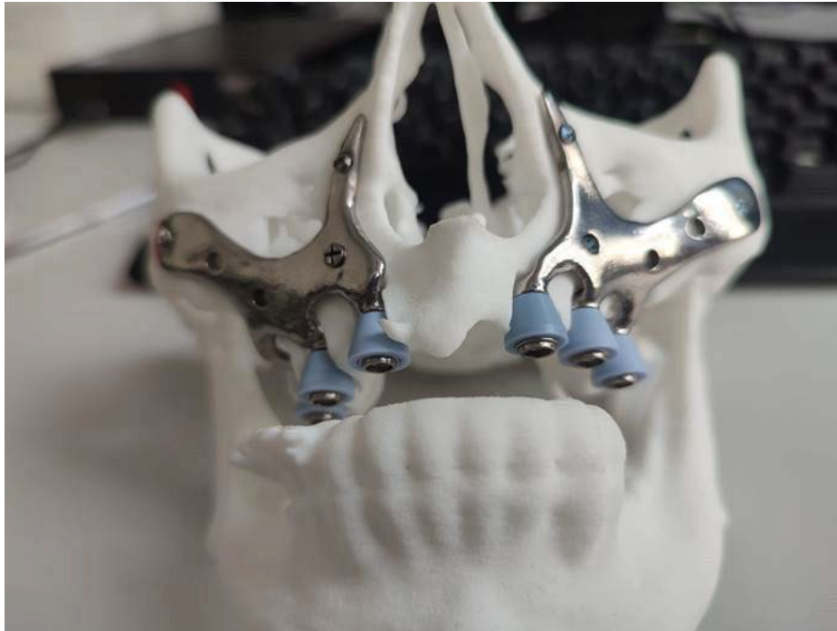
Figure 166: Image of 3D-printed model fitted with multi-material prosthesis, to illustrate proposed clinical application of the project
