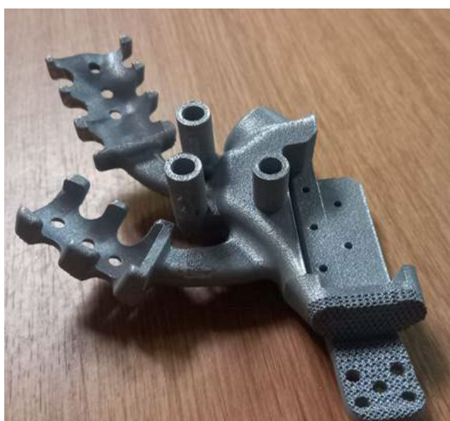
Figure 155: CAD design and titanium 3D-printed sternal implant manufactured for ATTRI
