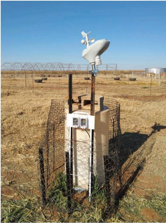
A setup of the smart farm which includes the WIFI weather station, soil moisture sensor as well a camera that works with WIFI.
