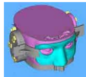
3D design of patient's skull, soft tissue and positioning mask completed by CRPM
