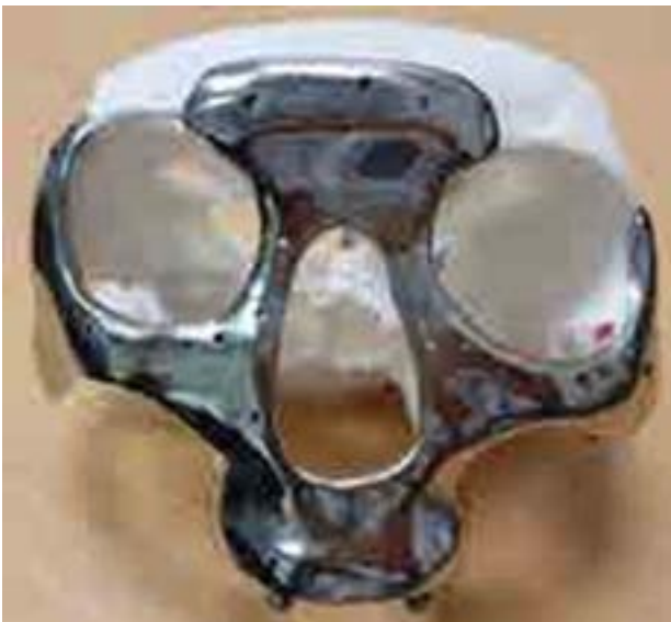
3D printed titanium implant after post processing
