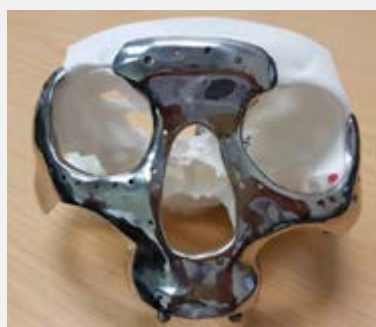
3D printed titanium implant after post processing
